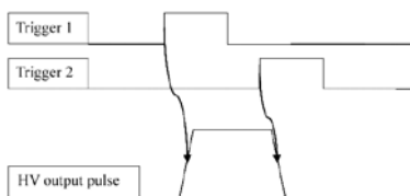
Fig. 1. Control timing charts for two-pulses controlled drivers
